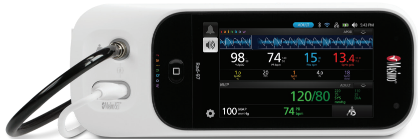
Rad-97 with Noninvasive Blood Pressure Integrated noninvasive blood pressure enables hospital-grade Pulse CO-Oximetry and vital signs monitoring in the home.
